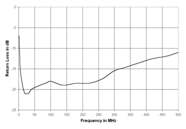
Figure 4 - Improved 4:1 Current Balun Return Loss
