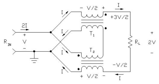
Figure 1 - The Guanella 4:1 Current Balun with Floating Load
