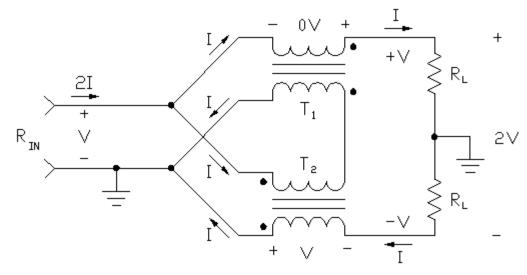
Figure 2 - The Guanella 4:1 Current Balun with Symmetrical Load
