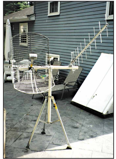
Fig 1.13 — Most communication with unmanned satellites uses VHF, UHF or microwave frequencies, and many hams build their own antennas for this pursuit.
